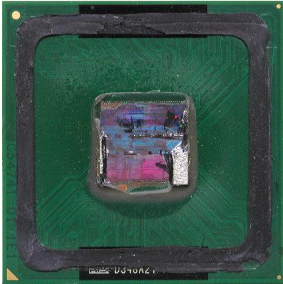
Pentium 4 with actual chip exposed
