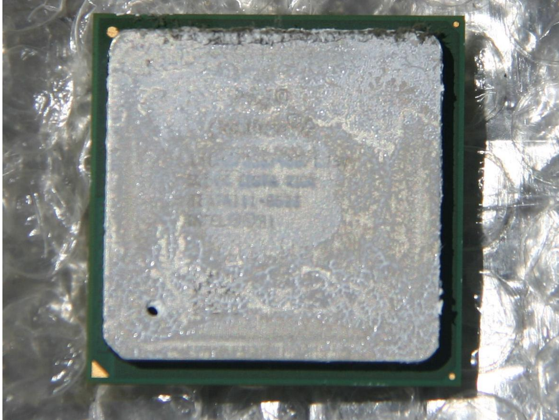
Pentium 4 CPU without heat sink
