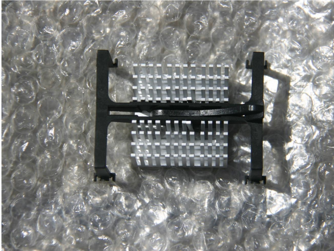
North Bridge Heat Sink
